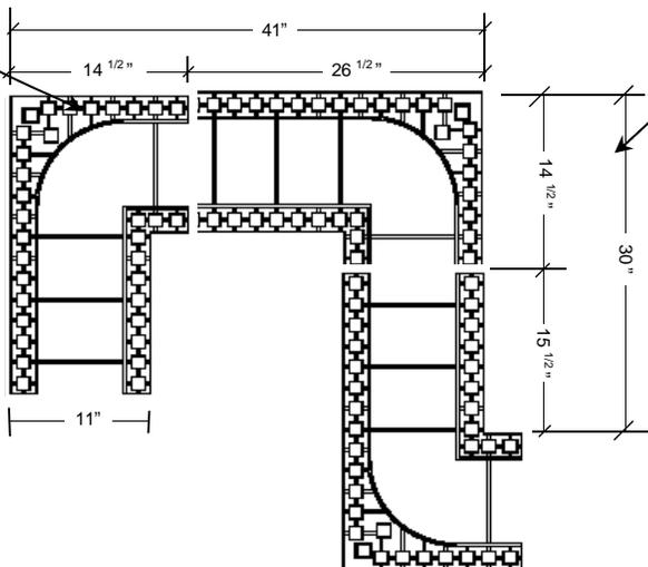
**Outside to Inside corners.** A minimum dimension that works to maintain an interlock is 30" (for 6-inch block). That provides the ability to create a running bond overlap between the blocks. Increasing the segment length by adding increments of 48" would keep a wall length that would not require any block cutting. Alternatively, incrementing from 30" in 6-inch increments would require block cutting, but still maintain zero waste.
